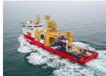
Spread Solution provided: 2000T demountable turntable, a loading tower with built in 15T tensioner and operators
