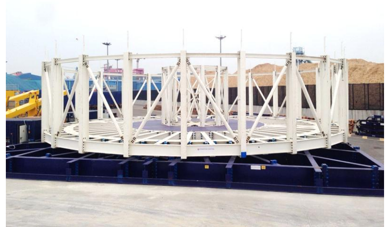
RentOcean's 4000T Turntable being built up at LS Cable quayside in South Korea
