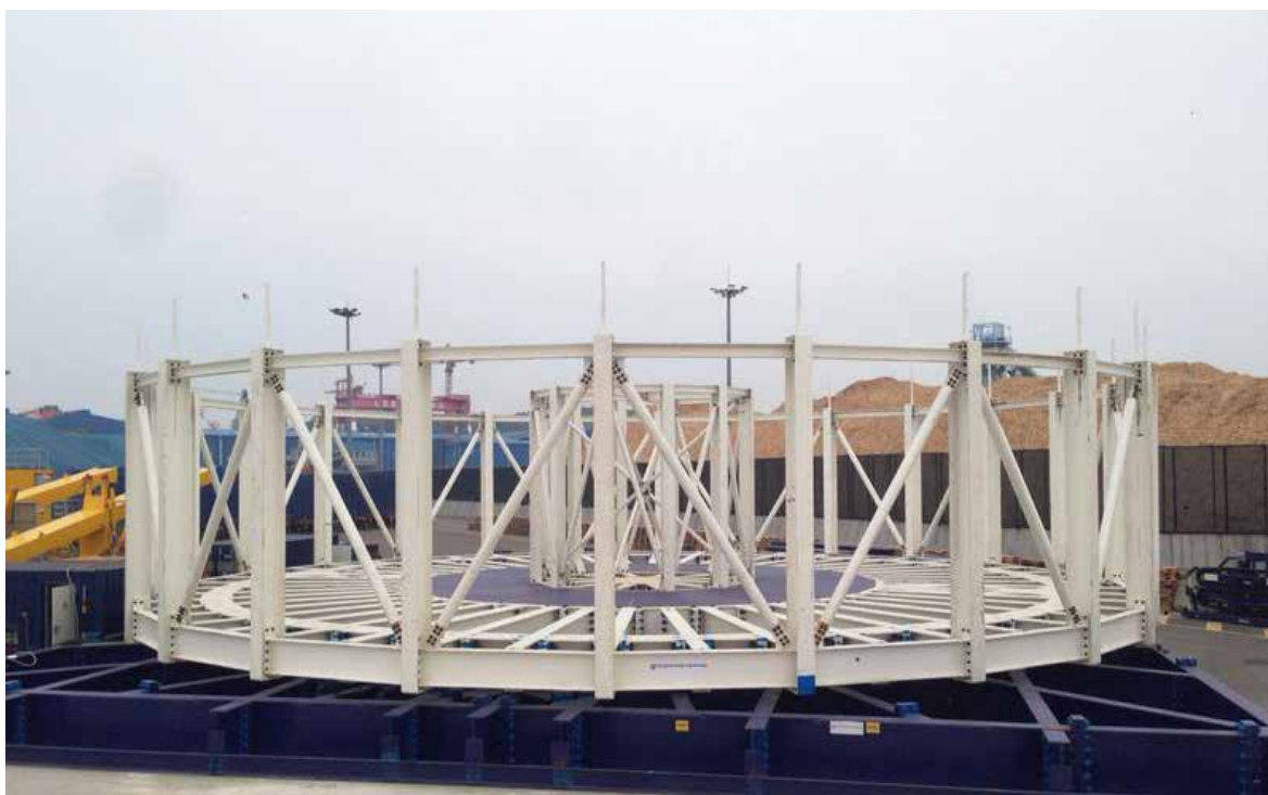
RentOcean's 4000T Turntable being built up at LS Cable quayside in South Korea
