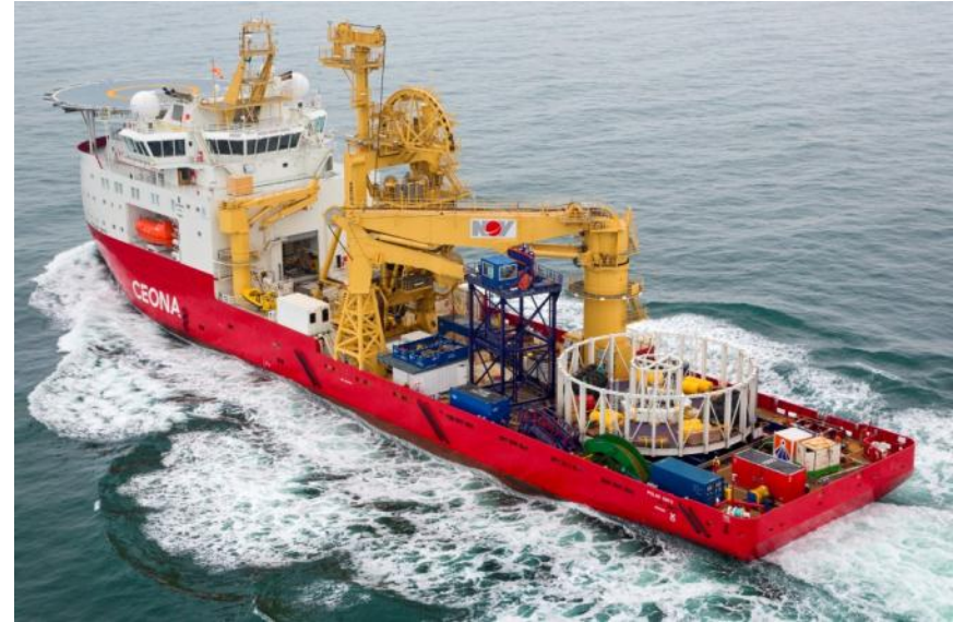
RentOcean's new 2000T modular carousel and loading tower with 15T tensioner on Ceona's Polar Onyx
