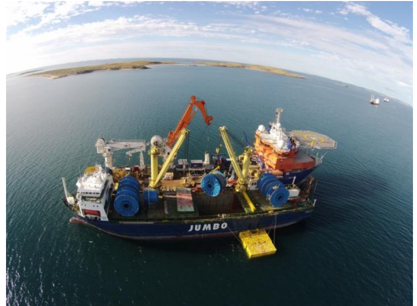
CSV Southern Ocean loading reels in North West Australia
