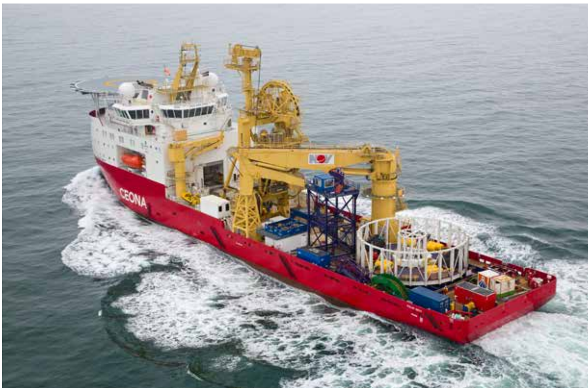
RentOcean's 2.000T Carousel and loading tower on Ceona's Polar Onyx.
