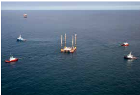
Relocation of KCI's own design multipurpose platform from P6-S to Q1-D for Wintershall.
