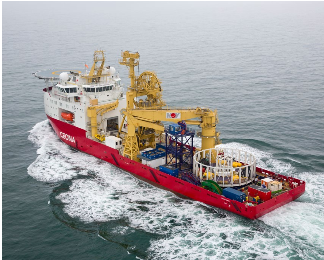
RentOcean supplied a modular 2000T turntable, loading tower with a built in 15T tensioner for a project in Brazil
