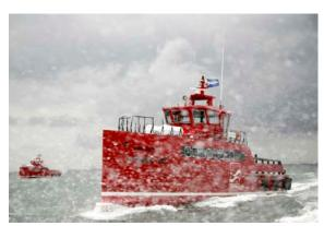
These innovative Fast Support Vessels (FSV's) are operational. The vessels are capable of transporting 75 p.o.b. and cargo at a cruising speed of 25 knots with largely improved fuel efficiency compared to similar vessel available.
