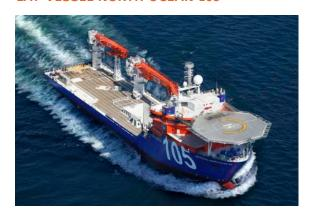
High-capacity, rigid-reeled vertical pipelay vessel, with 3000-ton payload reel capacity for subsea construction and installation, and deepwater moorings installation; which has been delivered the 20th April 2012. The vessel has started a five years charter contract at delivery.
