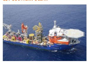
The vessel was delivered in Q4 2010 and immediately commenced its first project for Fugro TSMarine. This DP2 Construction Support / Flexible Product Installation vessel combines a moon pool, two large cranes (1 x 250tonnes and 1 x 110 tonnes, heave compensated), 2500m2 deck space, 120 accommodation and excellent seafaring capabilities, enabling her to be utilised for field support, construction, installation and IRM.
