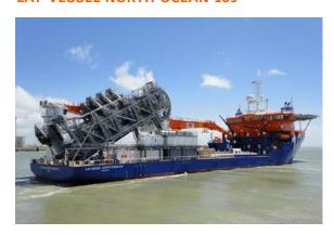
High-capacity, rigid-reeled vertical Pipe Lay Vessel, with 3000-ton payload reel capacity for subsea construction and installation, and deepwater moorings installation; which has been delivered the 20th April 2012. The vessel has started a 5 year charter contract at delivery.
