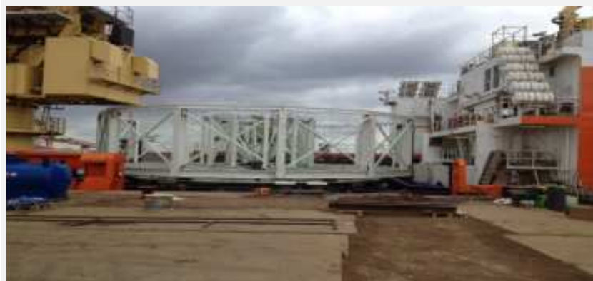
OTS 1250t modular turn table on board Normand Flower for VSMC
