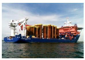
The vessel was delivered in Q4 2010 and immediately commenced its first project for Fugro-TSMarine Australia. This DP2 Construction Support / Flexible Product Installation vessel combines a moon pool, two large cranes (1 x 250tonnes and 1 x 110 tonnes, heave compensated), 2500m2 deck space, 120 accommodation and excellent seafaring capabilities, enabling her to be utilised for field support, construction, installation and IRM.
