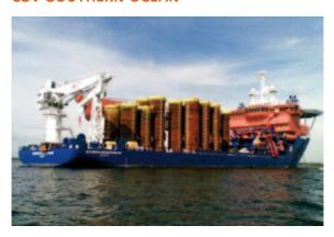
The vessel was delivered in Q4 2010 and immediately commenced its first project for Fugro-TSMarine Australia. This DP2 Construction Support / Flexible Product Installation vessel combines a moon pool, two large cranes (1 x 250tonnes and 1 x 100 tonnes, heave compensated), 2500m2 deck space, 120accommodation and excellent seafaring capabilities, enabling her to be utilised for field support, construction, installation and IRM.
