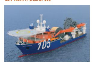
High-capacity, rigid-reeled vertical pipelay vessel, with 3000-ton payload reel capacity for subsea construction and installation, and deepwater moorings installation; which will be available as from Q2 2012 for installation works.
