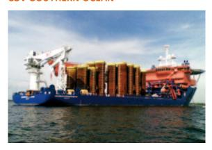
The vessel was delivered in Q4 2010 and immediately commenced its first project for Fugro-TSMarine Australia. This DP2 DP2 Construction Support / Flexible Product Installation vessel combines a moon pool, two large cranes (1 x 250tonnes and 1 x 100 tonnes, heave compensated), 2500m2 deck space, 120accommodation and excellent seafaring capabilities, enabling her to be utilised for field support, construction, installation and IRM.
