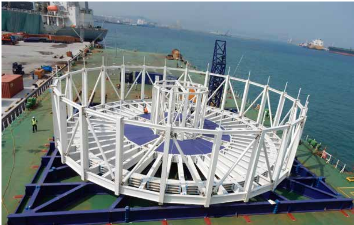
Our demountable 4000T turntable will be made ready for a cable laying project in Germany
