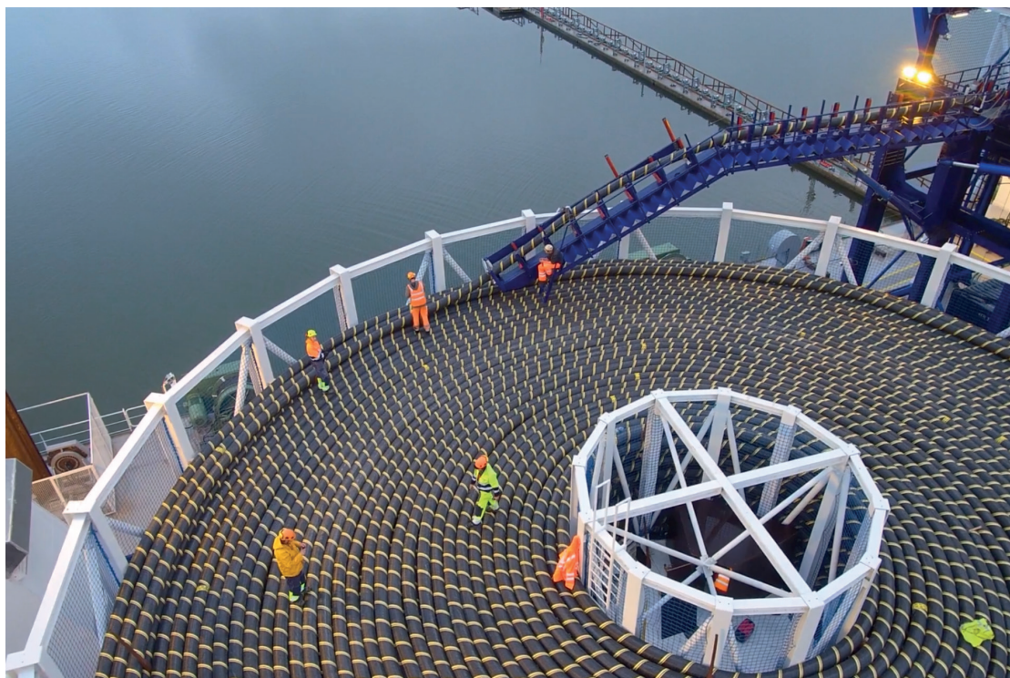
Spooling cable in Oceanteam's 4000Te carousel
